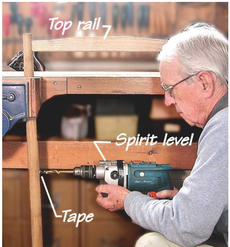
▲ Pic. 8 Getting down to drilling the lower back rail mortise holes
